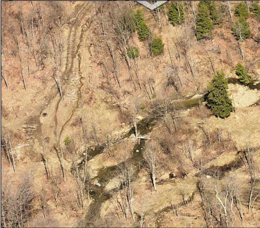
Figure 41. Erosion from Logging into Phelps Creek
